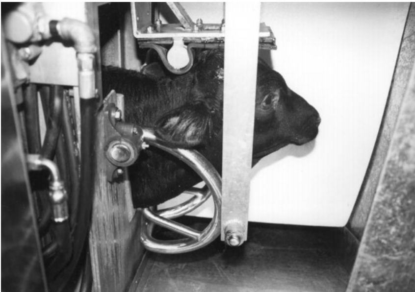
Fig. 3.12. A solid box around the animal's head will help to keep it quieter when a head restraint device is used. The box must be lit to induce the animal to place its head through the head opening.
